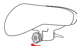
! Always use the knob for this adjustment! Moving the seat parts manually can damage the mechanism.
